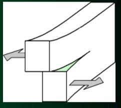
Mode I (Tension, Opening) Mode II (In-plane shear, Sliding)
