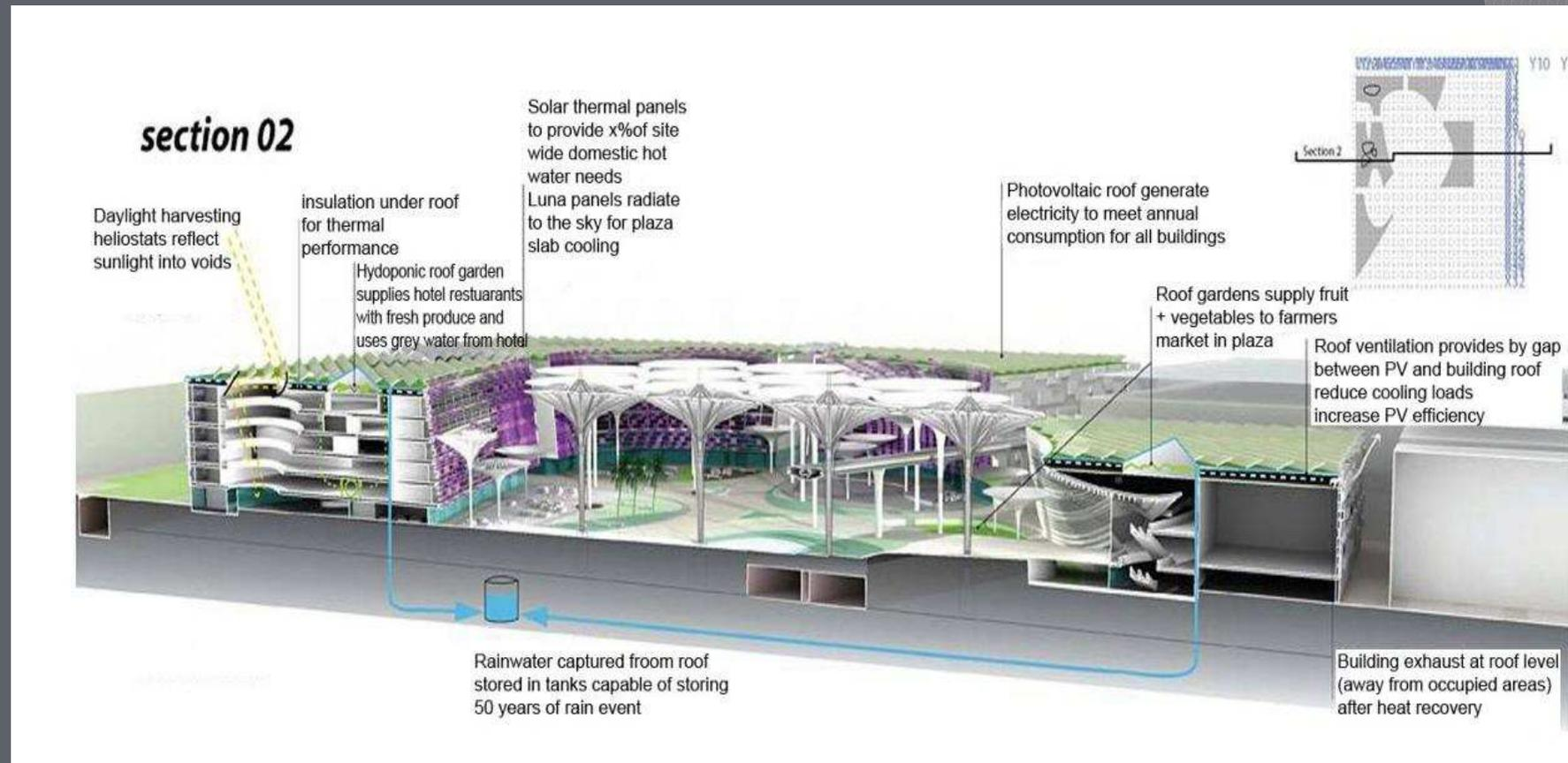
Fig. (14). shows cross sections demonstrating water flows to underground water tanks.
